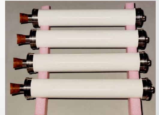
STAR-5D rocket motors used to decelerate Mars Pathfinder to zero velocity on the Martian surface
