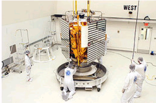
Technicians prepare MESSENGER for transfer to a hazardous processing facility prior to loading the spacecraft's complement of hypergolic propellants.
