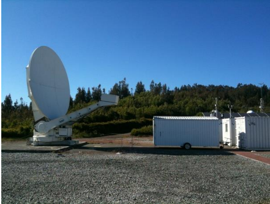
A radio telescope with a cryogenic dual band S/X-band receiver (TIGO, Concepcion, Chili)
