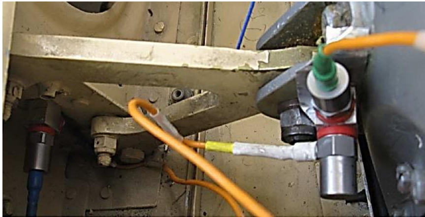
Bolted connection between wing tip and fuel tank.
