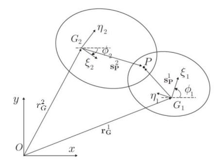
$$\overline{r}_G^1 + A_1 \overline{s}_P^1 = \overline{r}_G^2 + A_2 \overline{s}_P^2$$
