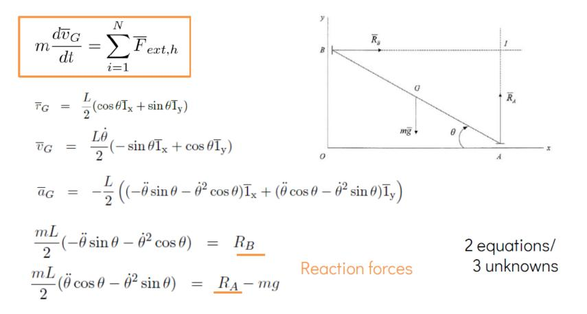
Choice of I allows to get rid of reaction forces  $\rm R_{A}$  and  $\rm R_{B}$
