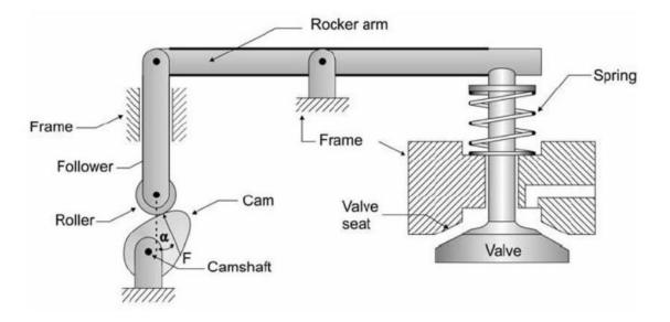
Kinematical analysis : satisfy functional requirements for valve displacements.
