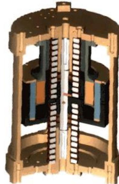
Sealed cylinder with a disc sandwiched between 2 coil springs
