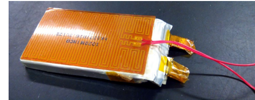
OUFTEI heater on the battery
