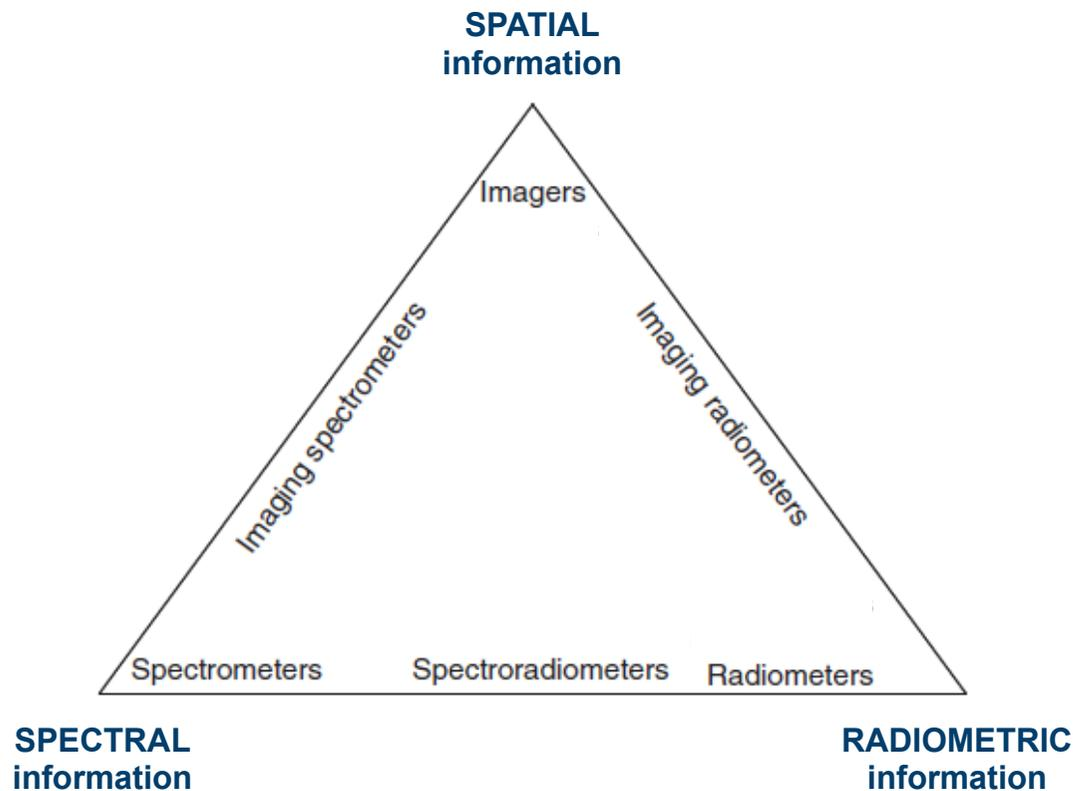
Diagram illustrating the different types of information and the type of sensor used to acquire this information
