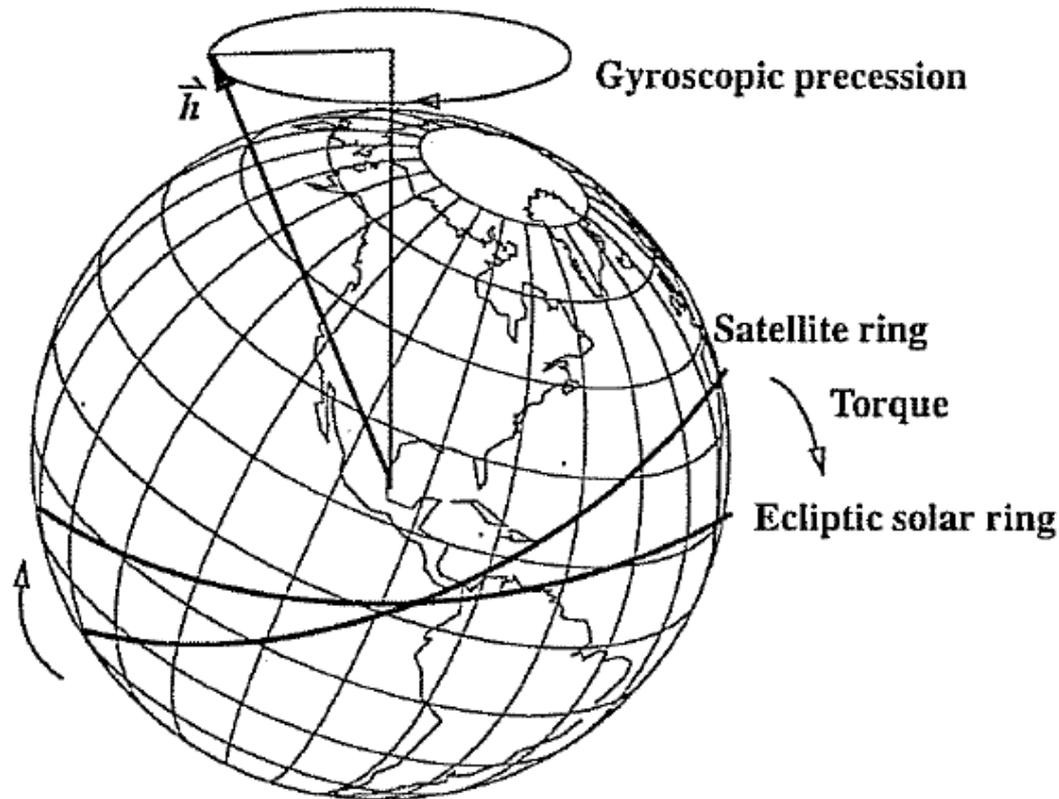
The Sun's attraction tends to turn the satellite ring into the ecliptic. The orbit precesses about the pole of the ecliptic.
