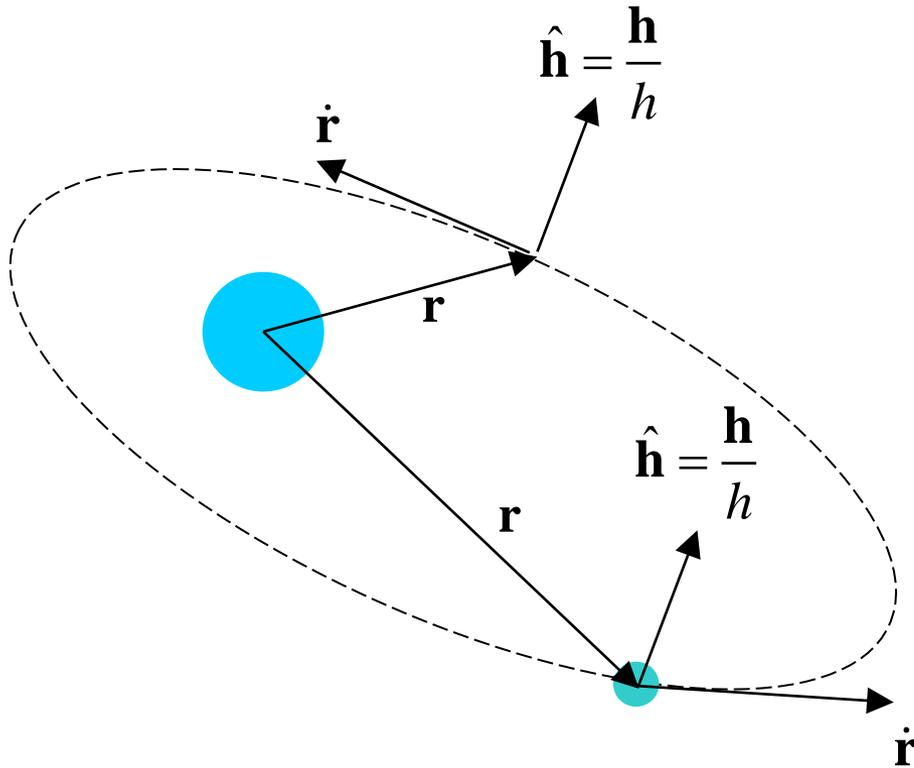
The fixed plane is the **orbit plane** and is normal to the angular momentum vector.
