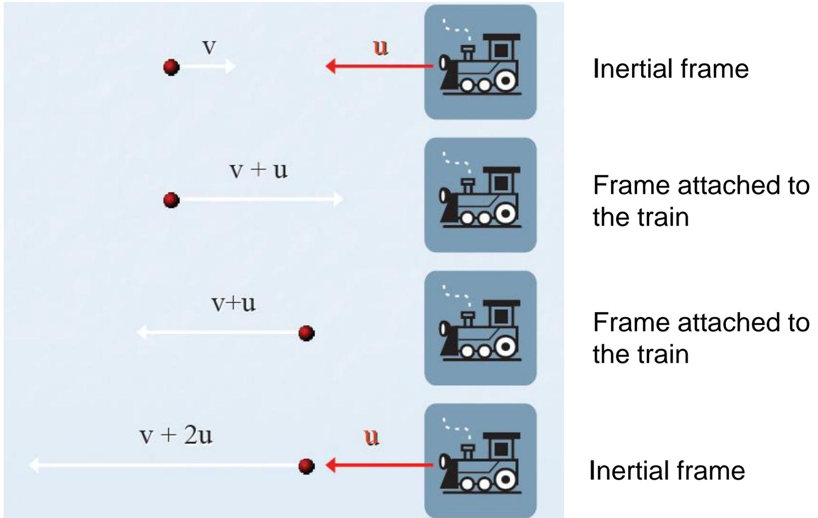
A gravity assist looks like an elastic collision, although there is no physical contact with the planet.
