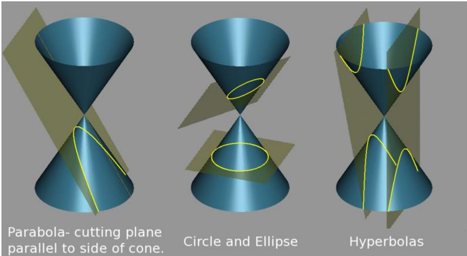
Parabola- cutting plane parallel to side of cone.
