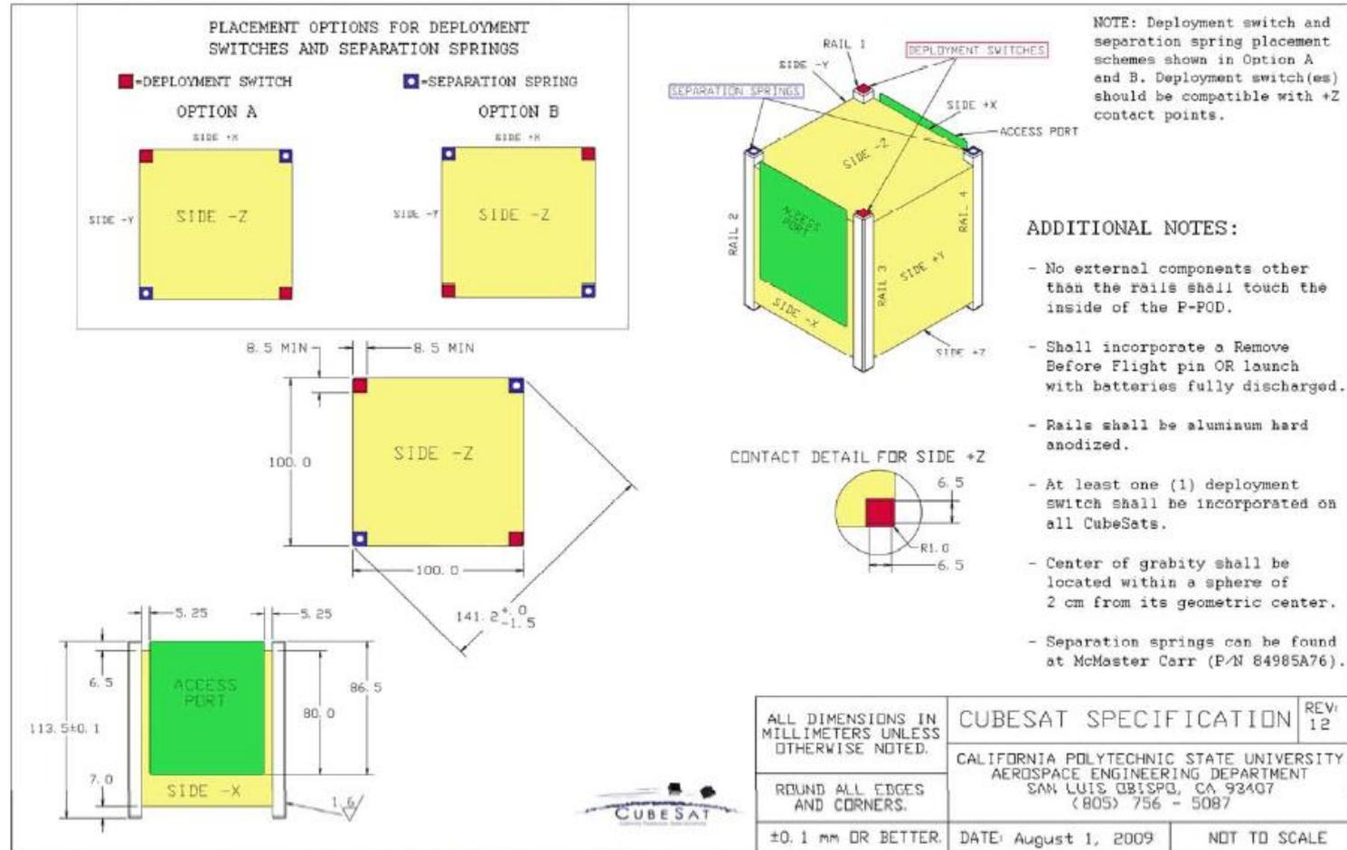
Figure 5: CubeSat Design Specification Drawing
