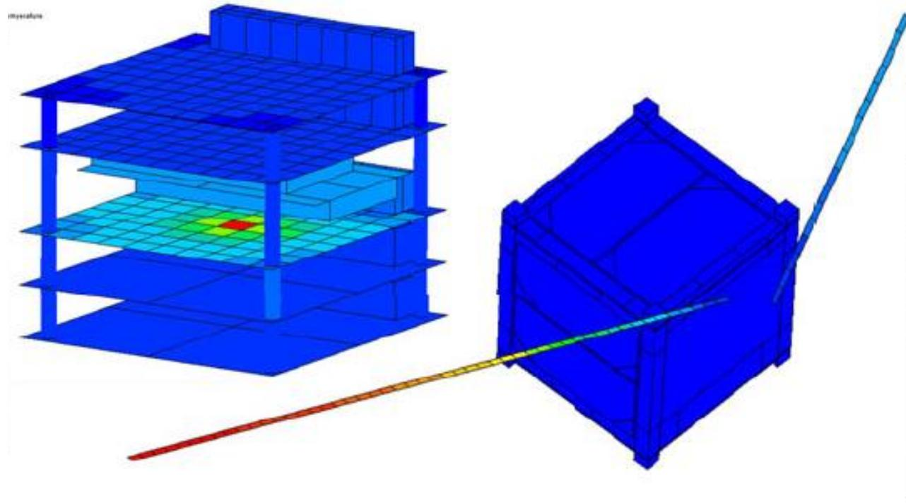
Hot spot due to dissipation transistor !
