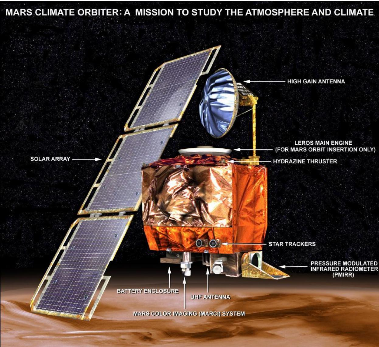
Due to a navigation error, Mars Climate Orbiter was lost. The error arose because Lockheed Martin used imperial units instead of metric units as specified by NASA
