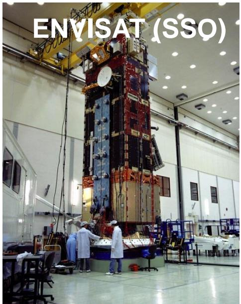
In-orbit configuration: 26 m x 10m x 5m
